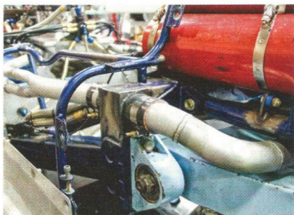
[Cooling lines are new and snake throoughtout the frame. Again, changes required modifications that can be seen in bare metal. The chassis will be disassembled and painted and detailed before being reassembled.
