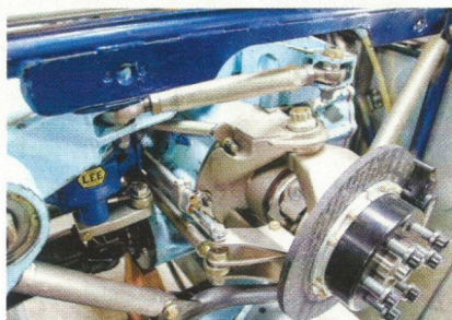
[Fabricated knuckles and massive U-joints replace the stagecoach-steering. The original '68 Camaro box from Lee MFG was retained.]
