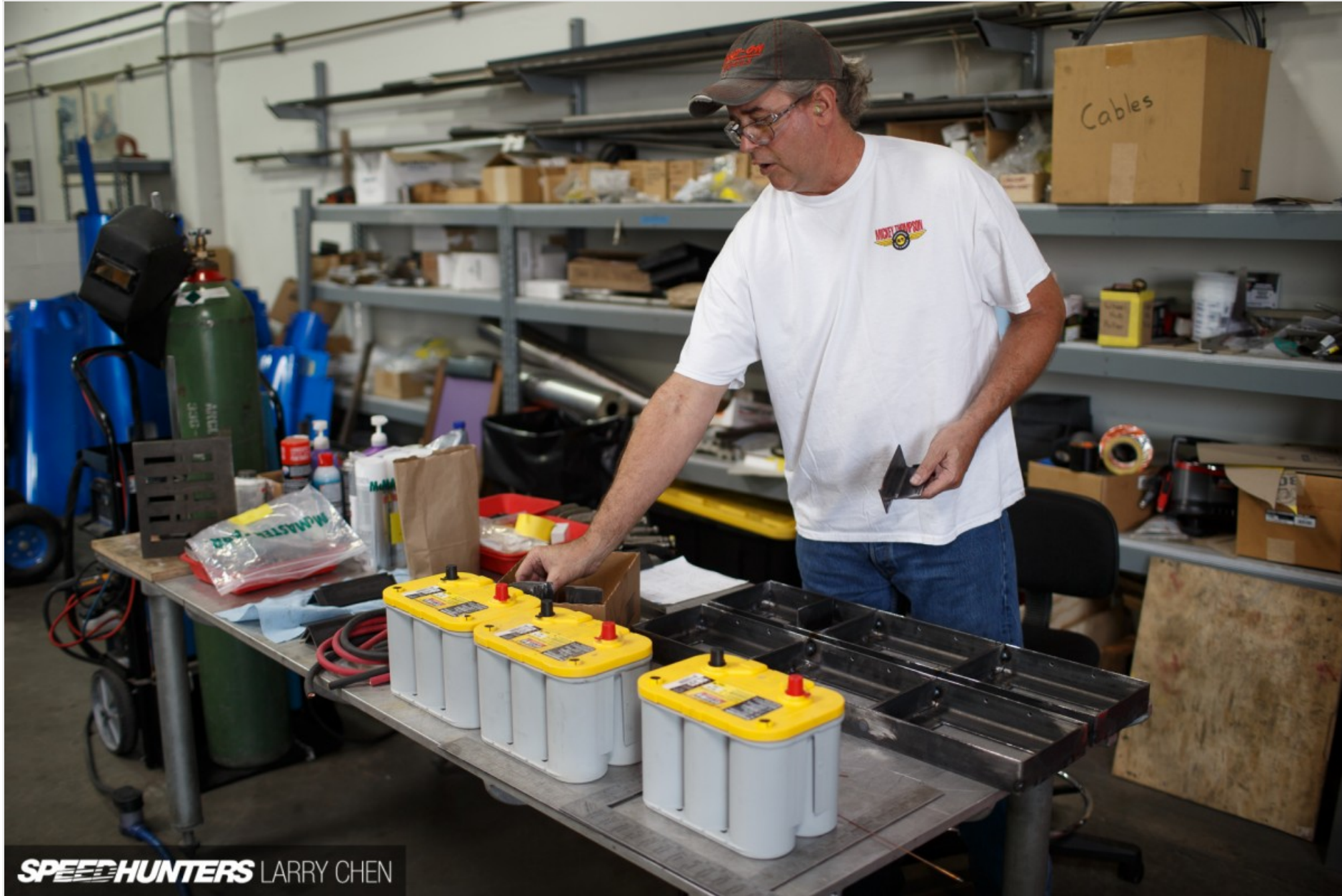
Other last minute details include fabricating a starter cart that houses three Optima yellow top batteries. This will be used to spin the starters on the line, then unplugged and moved away.
